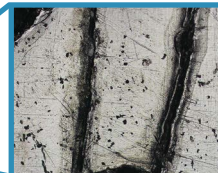
Crack in threaded hole UV irradiation photo
