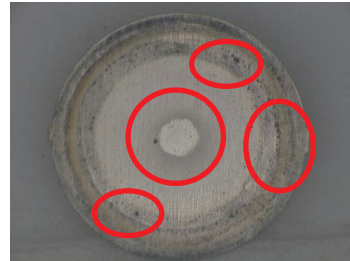
Dusts adhere to the contact surface, and it causes a contact failure
