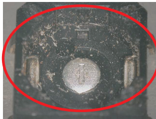
Dusts enter through a gap between the plunger and the cover
