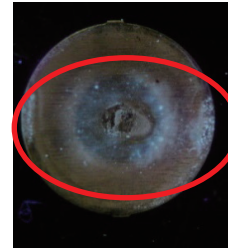
Flux adheres to the contact surface, and it causes a contact failure
