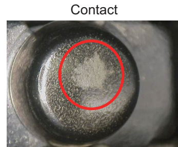
Contact Flux adheres to the contact surface
