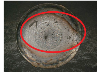
Dusts adhere to the contact surface, and contact failure results
