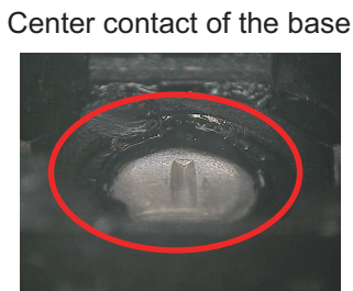
The resin around the contact is puffed up because it is melted, so it doesn't work properly
